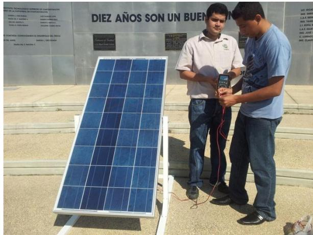
Fig. 2. Panel Solar ERDM 135SP6 de 135W a 20V.
