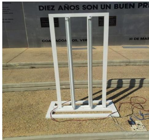
Fig. 10. Lámparas Led's T-8 de 20 Watts.
